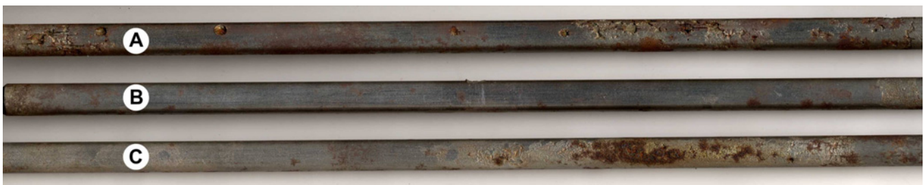
FIGURE 10: Surfaces of dismantled rebars (after pickling of the corrosion product)
