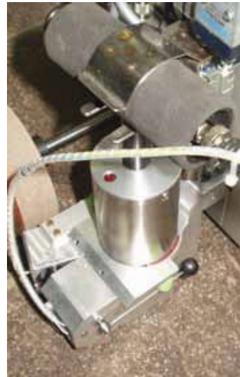
A close up view of the DOCter transducer and one of the two spherical impactors
