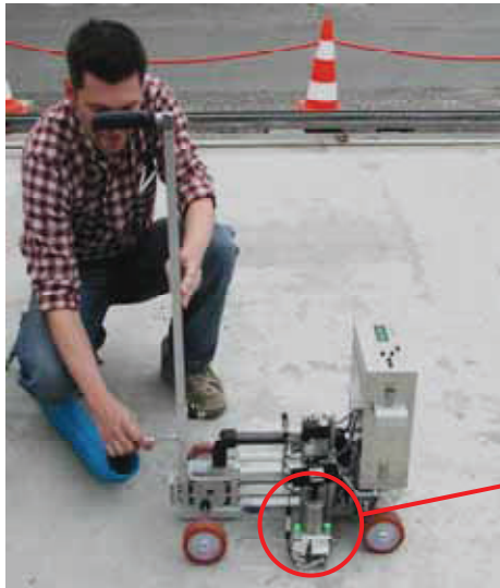
The STEPPER unit contains an electrical drive system for automated scanning and a pneumatic system for automated testing
