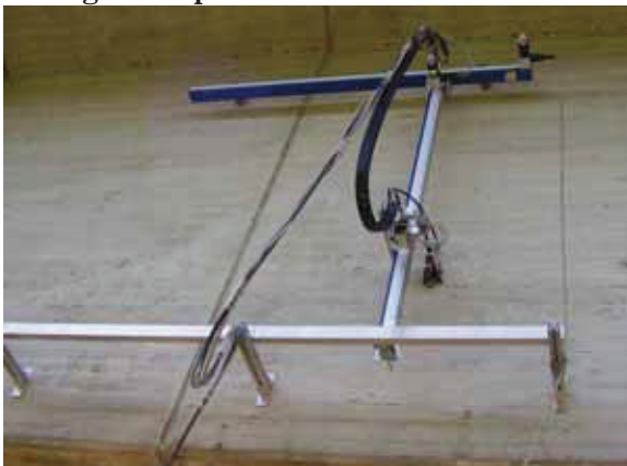
Vertical wall scanner system attached to web of post-tensioned bridge
