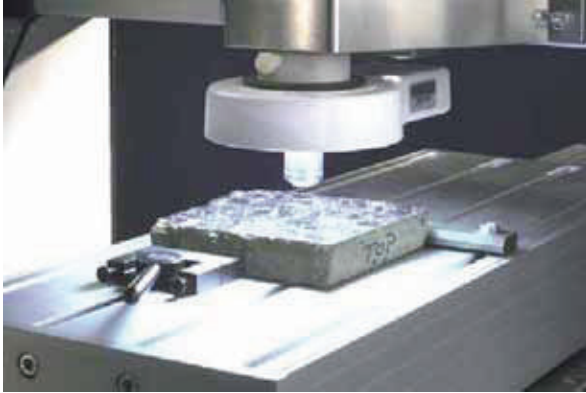
Prepared specimen positioned on the moveable stage ready for image analysis.
