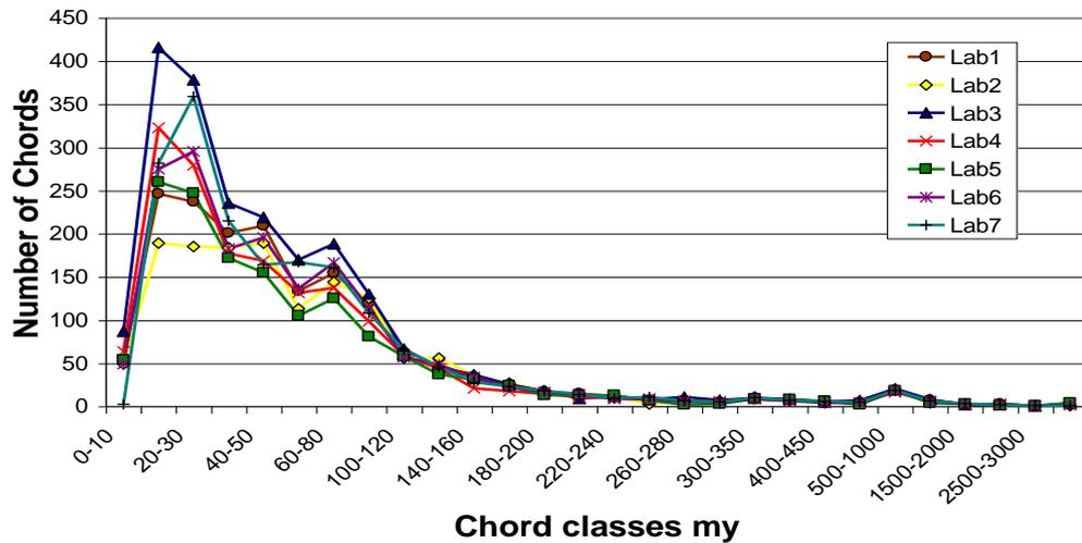
Figure 9: RapidAir chord length distribution determined by 7 laboratories.
