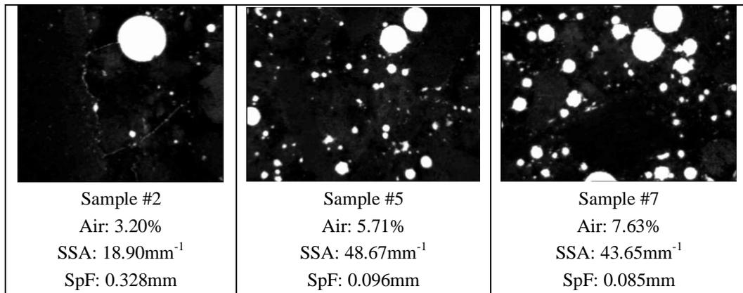
Figure 6: Close-up of the air void structures of the samples analysed. The images were collected during analysis. The average results of the automatic analysis are provided below the images (from Tables 2, 3 & 4). Abbreviations: SSA: specific surface area, SpF: spacing factor
