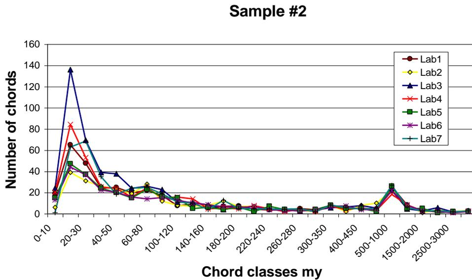
Figure 8: RapidAir chord length distribution determined by 7 laboratories.
