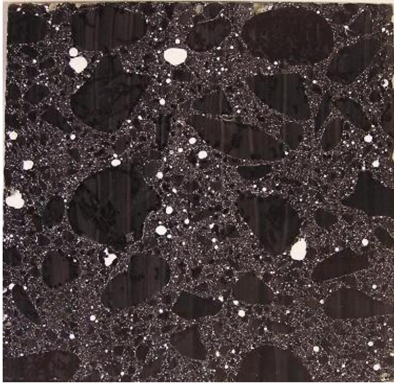
Figure 3: Appearance of sample #5 after being coloured black and white BaSO<sub>4</sub> powder filled into the air voids.
