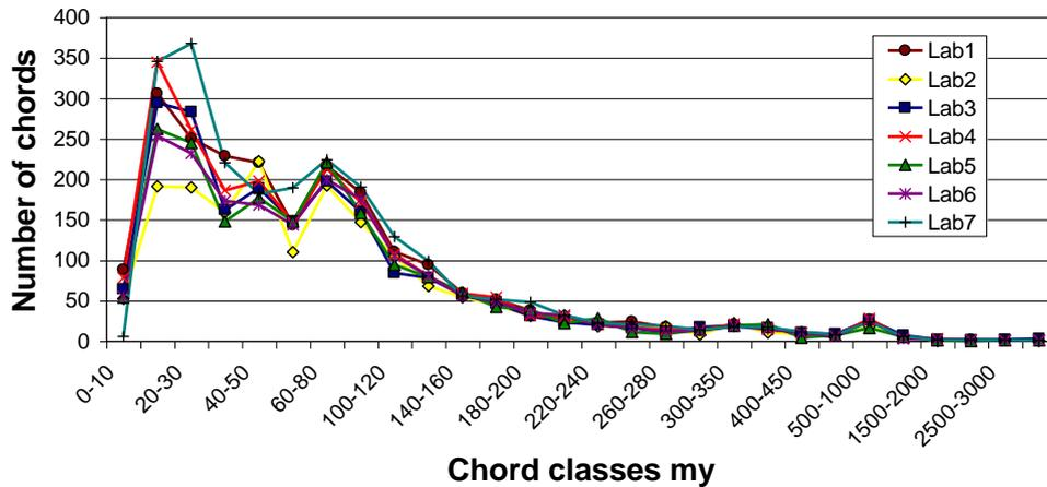
Figure 10: RapidAir chord length distribution determined by 7 laboratories.
