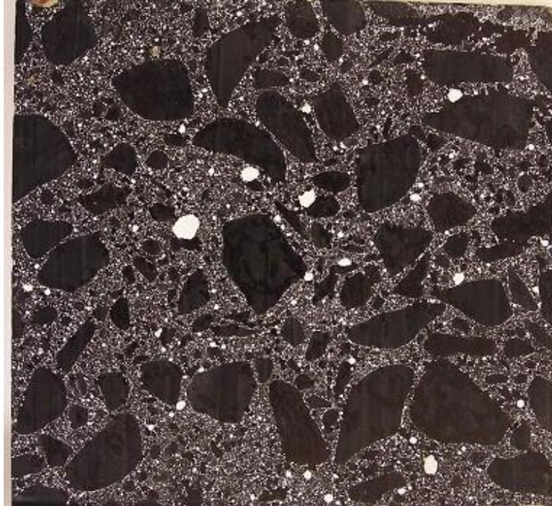
Figure 4: Appearance of sample #7 after being coloured black and BaSO<sub>4</sub> powder filled into the air voids.
