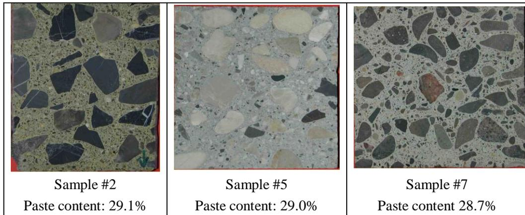
Figure 1: Appearance of the lapped samples. The manually determined paste content of the samples is noted below the images.
