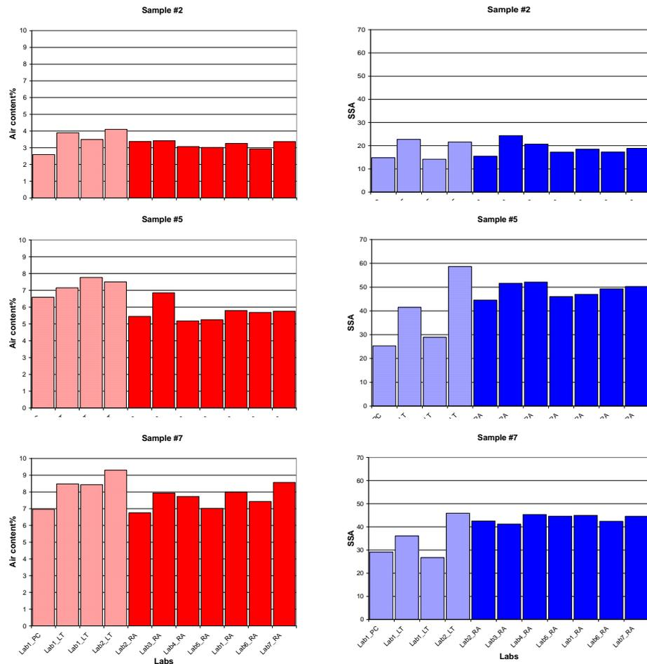
Figure 7: Graphical presentation of the air content and specific surface area (SSA) of the 3 samples analysed. Hatched: manual readings, solid: automatic analysis
