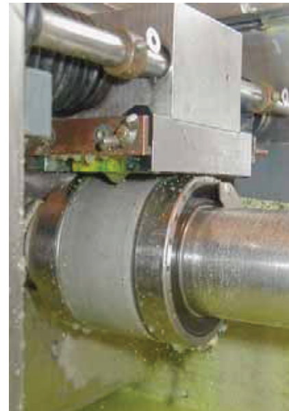
Grinding roller and massive sample holder in operation
