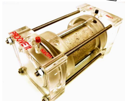
PR-1200 cell adapted for high length specimens when performing ASTM C 1760
