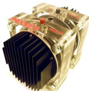
Special PR-1100 cell with cooling ribs. An option to control the heat produced in specimens of highly permeable concrete
