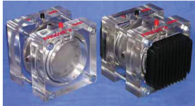
Two types of PROOVE'it cells: standard PR-1000 cell (left) and PR-1100 cell with cooling ribs (right)
