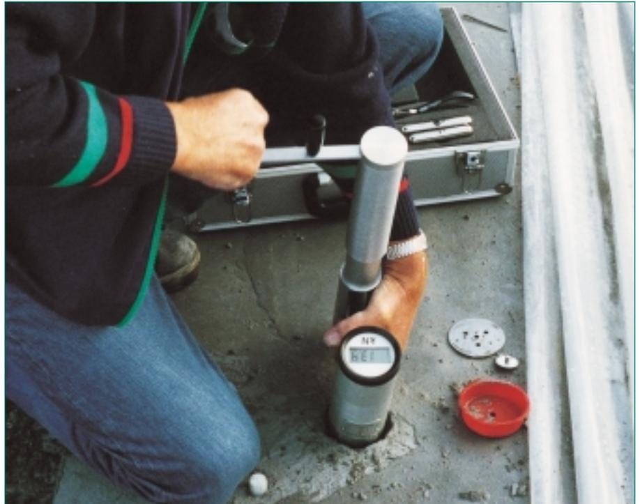
**Figure 1:** the Lok-test jack in position.
