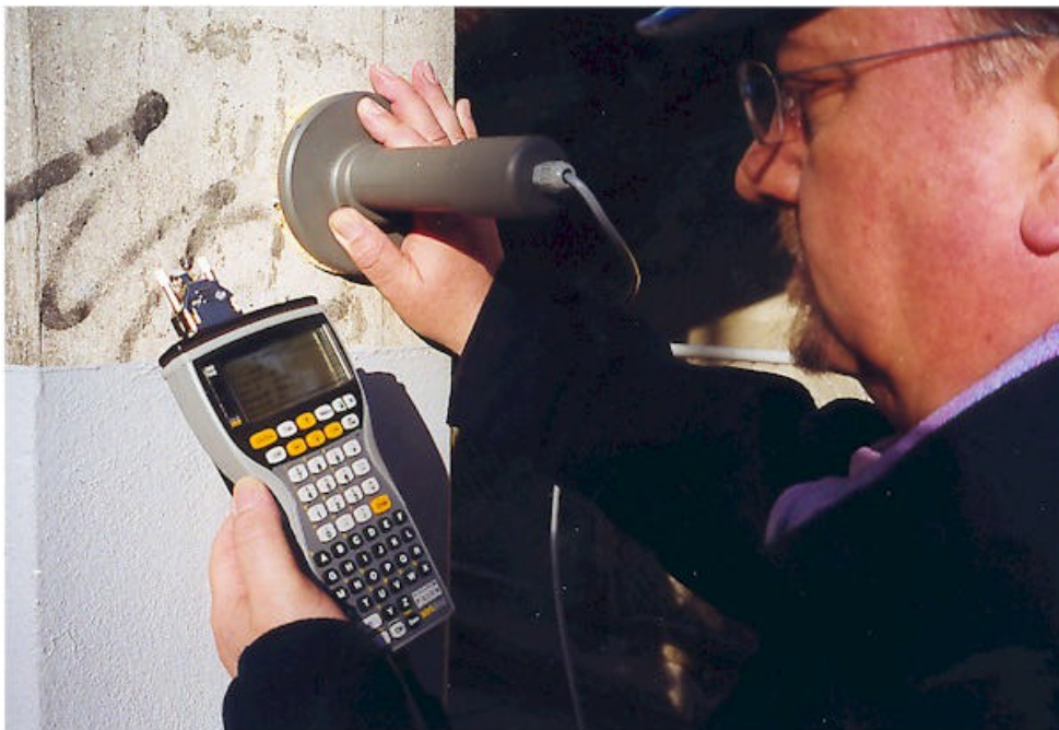
Fig. 1. Testing with the GalvaPulse in progress, on site.
