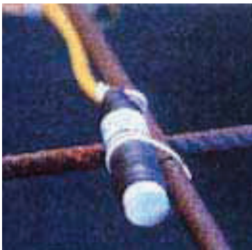
The ERE-Probe attached to reinforcement before placing concrete
