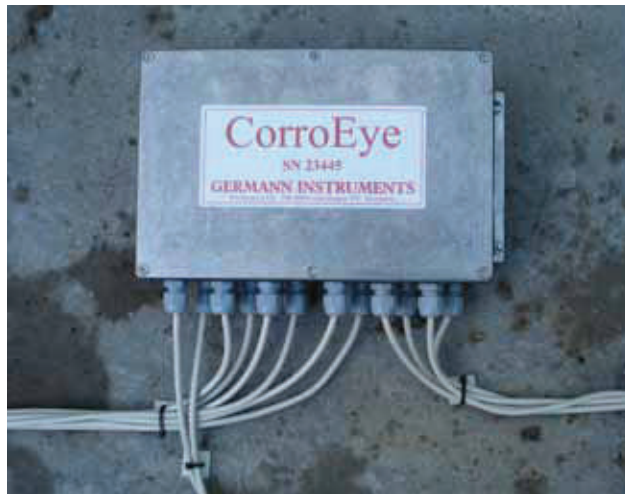
The CorroEye pulse generator and data logger unit
