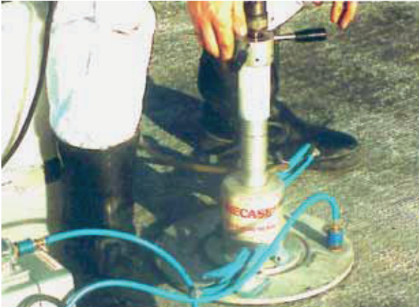
The CS-75 coring rig attached to the suction plate before conducting BOND-TEST
