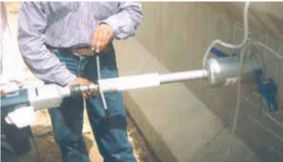
Coring with the CEL-100 rig to obtain specimen for testing with PROOVE'it for chloride permeability
