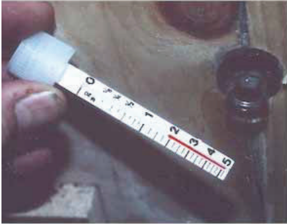
Maturity measured by the COMA-Meter before in-place strength testing with LOK-TEST for early form removal.
