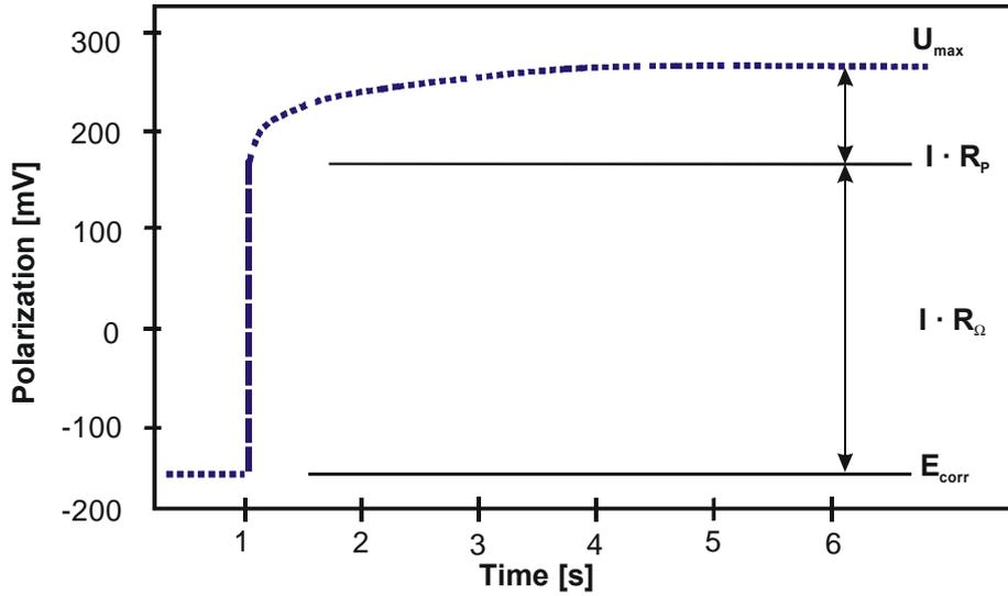
Fig. 1. Typical polarisation pattern
